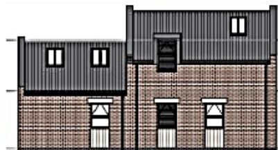
4. Side elevation showing 'Stepped' design to reduce impact on No.3
